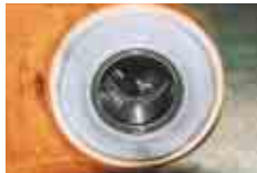
WC (Tungsten Carbide) Thermal Spraying
